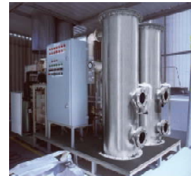
CE-100 Evaporator treating water contaminated with herbicides
